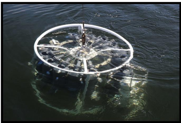
King County's conductivity-temperature-depth (CTD) profiler pictured above, which is lowered through the water from the boat. It measures water quality parameters throughout the water column and collects water samples for laboratory analysis.
