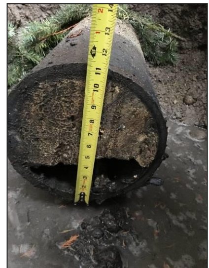
Section of pipe filled with fat and debris, Lake Hills Siphon
