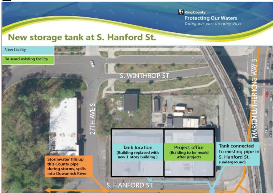
Figure 12. Rainier Valley Wet Weather Storage Project New Storage Tank
