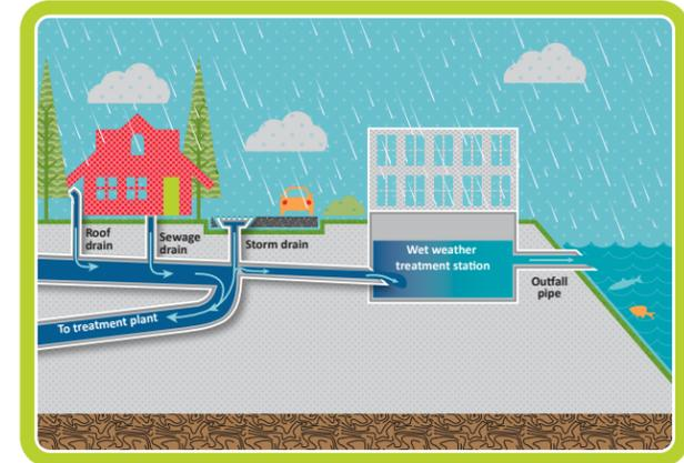
In Georgetown, King County will build a wet weather treatment station to help protect the Duwamish River from CSOs. During heavy rainstorms, the new station will clean excess sewage and stormwater before it enters the Duwamish River. The new facility will reduce the amount of untreated wastewater entering the Duwamish by 95 percent.
