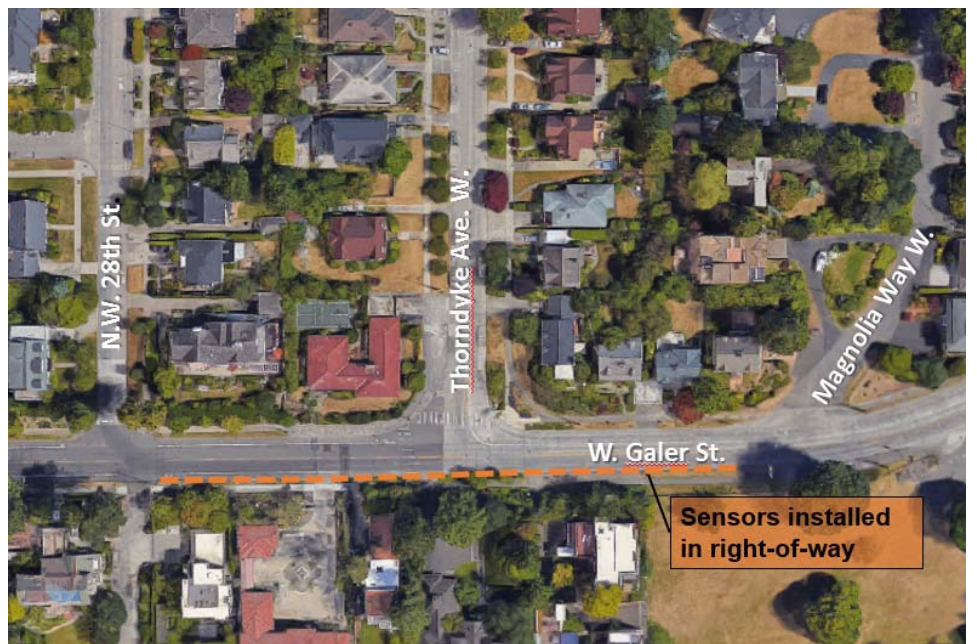
King County crews will install sensors in the W. Galer St. right of way this week to evaluate potential soil loss above a damaged County sewer pipeline 150 feet below the surface.
