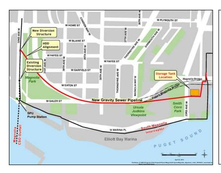
The new gravity sewer pipeline will stretch from 32<sup>nd</sup> Ave. W. to a new 1.5 million gallon underground storage tank near Smith Cove/Terminal 91. This facility will store peak combined sewer flows so that discharges of untreated wastewater and stormwater into Puget Sound are limited to no more than one per year on a long-term average.
