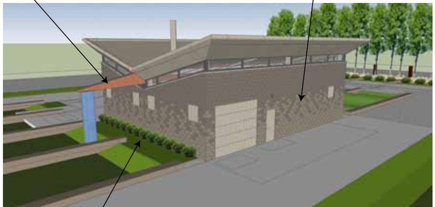
Sidewalk replaced with low vegetation to soften profile and prevent splashing onto building
