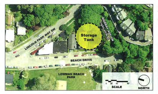
The tank will store sewer and stormwater overflows during storms – keeping them out of Puget Sound. A circular tank reduces construction impacts for the community.
