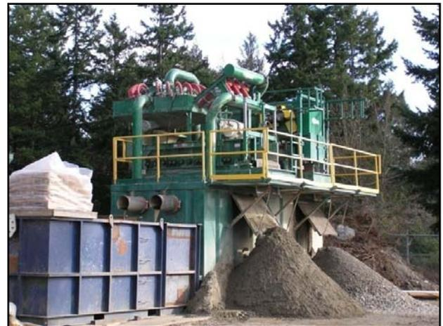
*A slurry separation plant is used to process excavated soils from the microtunnel*
