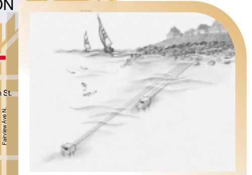
Two new outfalls will be installed at the Denny Regulator in Myrtle Edwards Park. One outfall is 500 feet offshore and 60 feet deep; the other is 100 feet offshore and 20 feet deep. The existing overflow at the shoreline will be removed.
