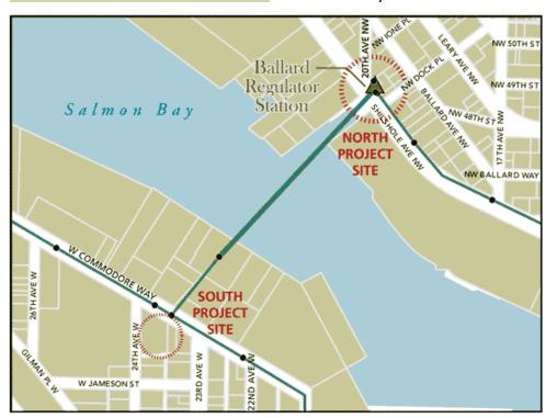
Wastewater from homes and businesses in Ballard now flows through the 36-inch siphons and across the bay, moving from the higher elevated pipes on the north side of the canal to the lower elevation on the south side, for treatment at the West Point Treatment Plant in Magnolia.
