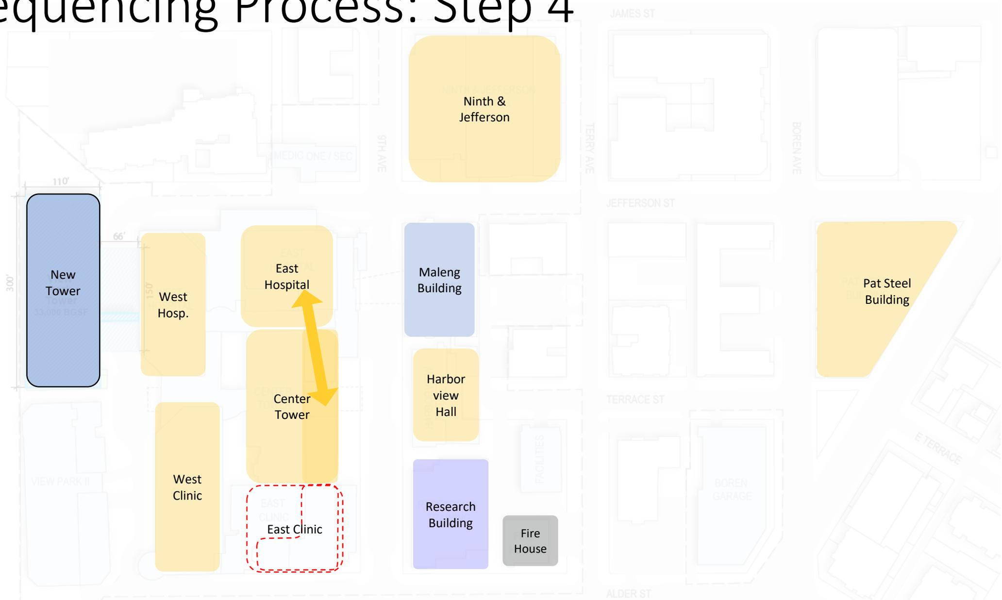
Demolish East Clinic/Seismically renovate Center Tower, decanting into East Hospital 3 floors at a time
