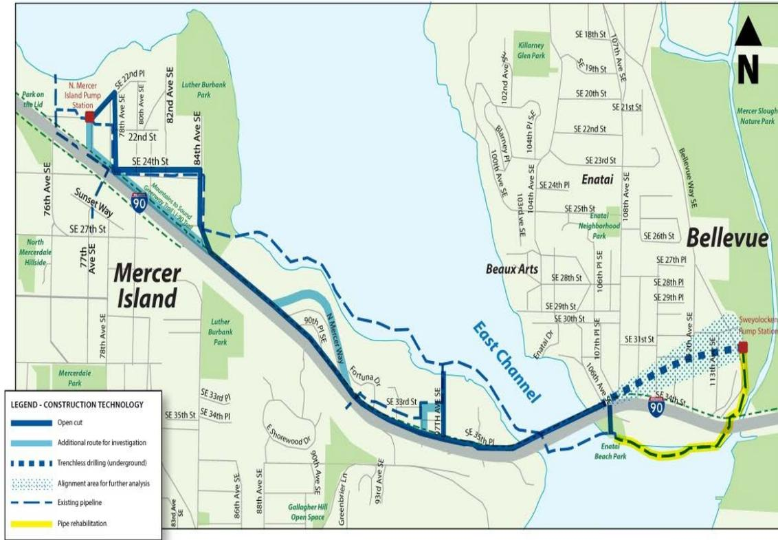
Figure 4. North Mercer Island and Enatai Sewer Upgrade Project Recommended Alternative
