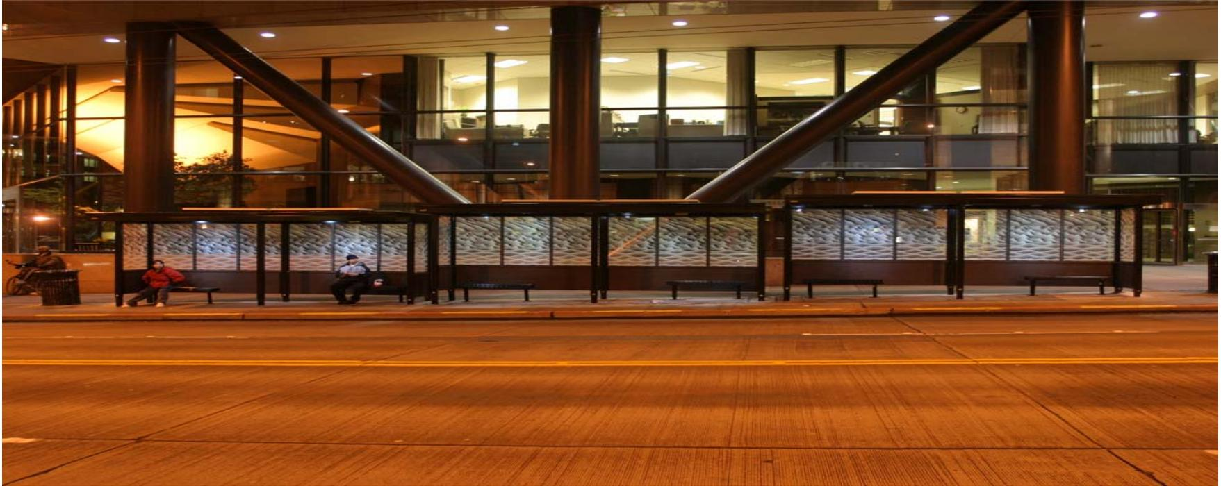
The past several years Power and Facilities has been installing solar powered LED (light emitting diodes) light fixtures. This technology uses PV (photo voltaic) arrays mounted on the roof of the shelter which charge a battery pack during the daylight hours and then the batteries power the LED fixtures during the night. This technology is working very well and we are committed to its continued use in the future.
