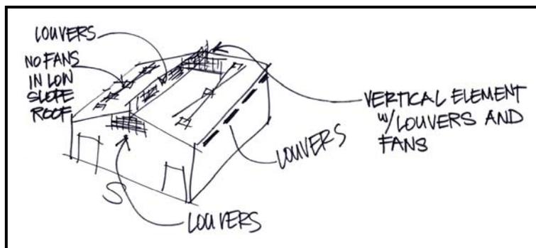
**Fig 3. Axonometric sketch of inlet/outlet locations on the building envelope**
