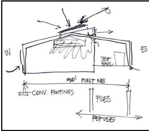
**Fig 2. Transfer Station section with overhead daylighting**
