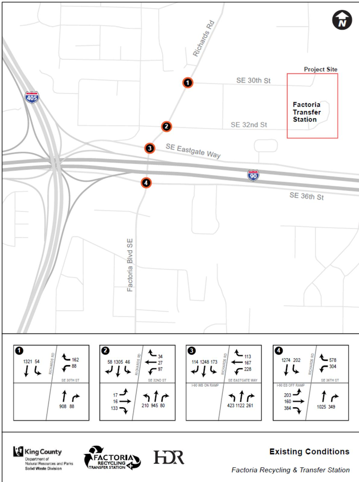
Figure 2-2. Existing PM Peak Hour Turning Movement Counts
