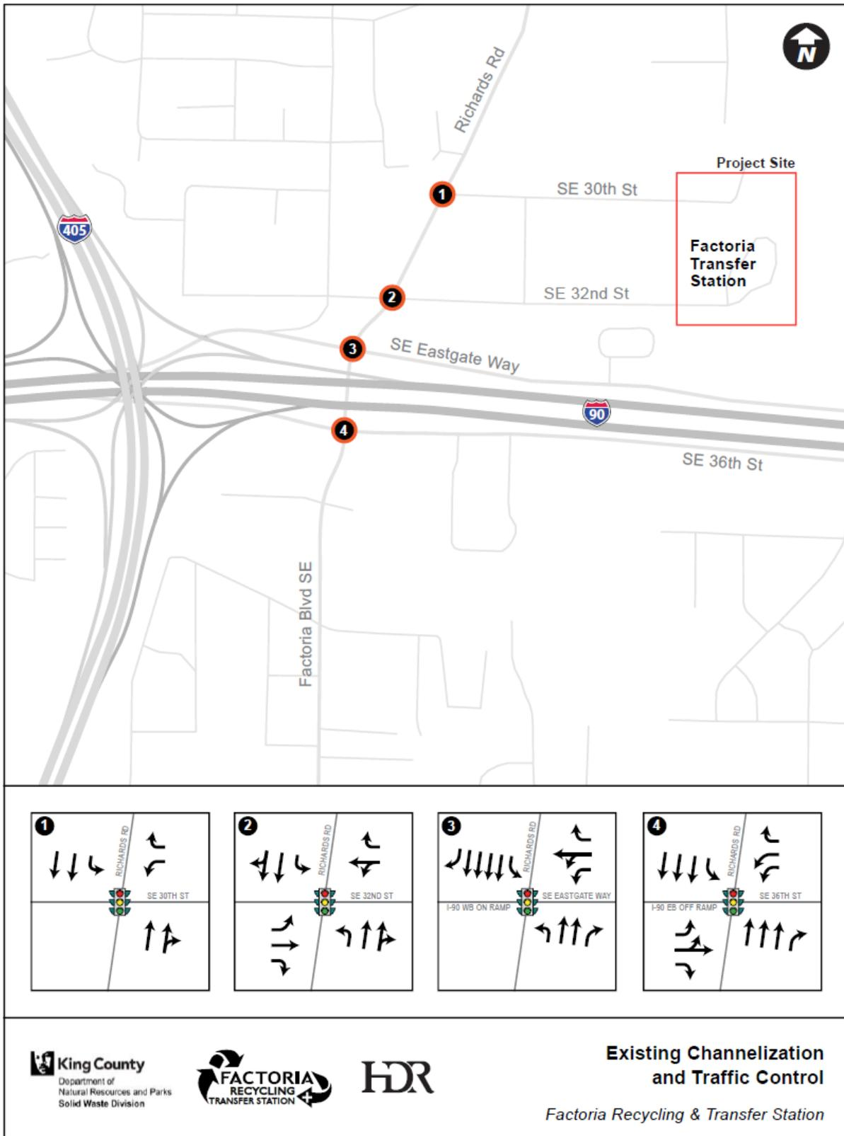
Figure 2-1. Existing Channelization and Traffic Control
