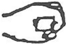
**TIP GRASP:** Engaging the PP 1 air brake valve with 2 or 3 fingers with up to 7 lbs. of force.
