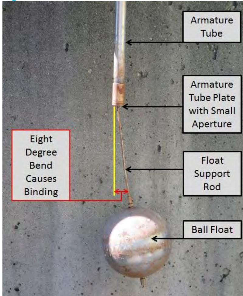
In addition, the bent support rods would most likely cause the float ball to rub up against the inside wall of the stilling wells, creating additional friction and requiring even more force for the rod to move up.
