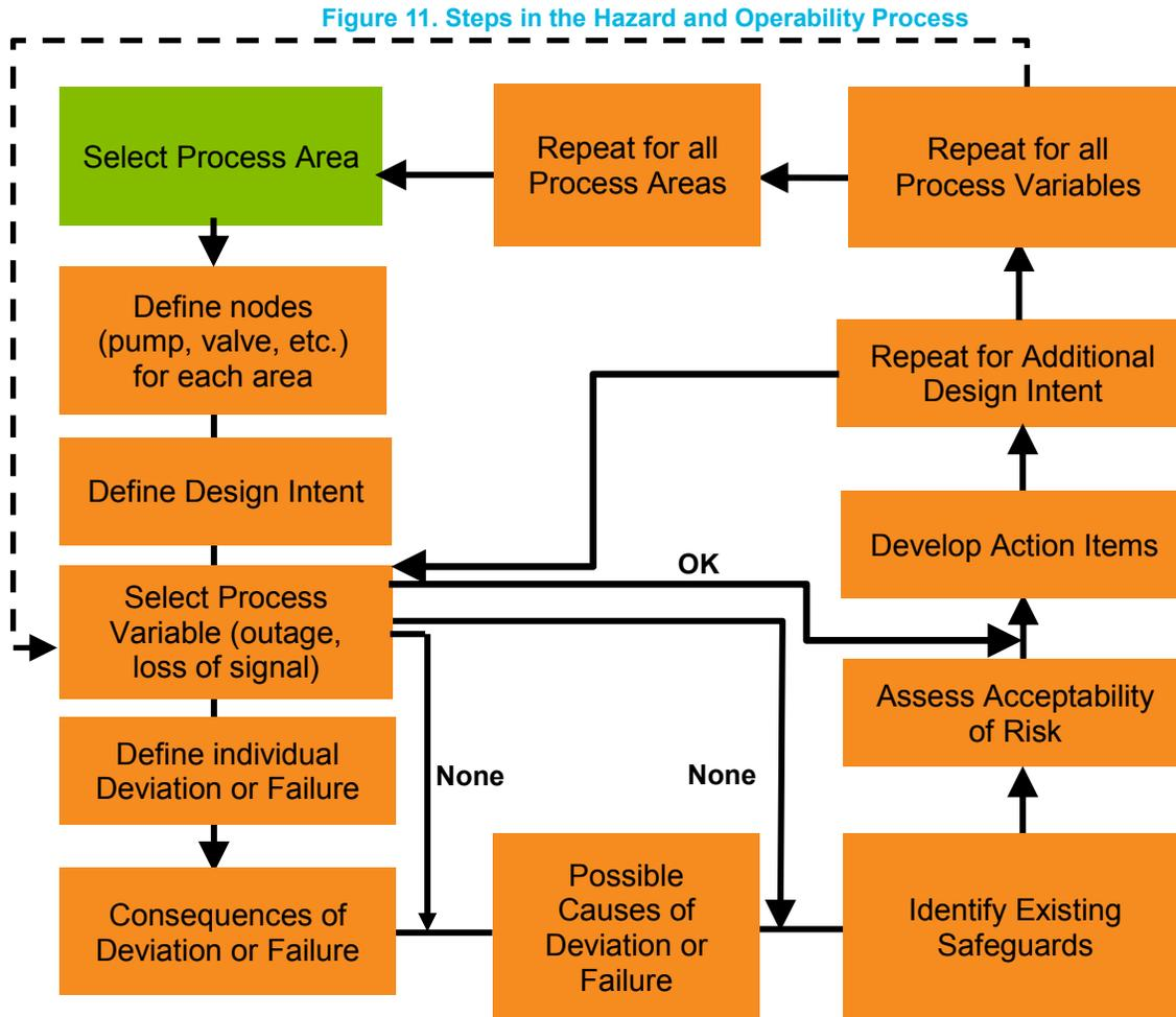
For this evaluation at WPTP, AECOM limited the HAZOP analysis to process-critical components that would cause a flood at the plant if operational failure were to occur. The following components of the plant were considered critical unit operations and processes:
