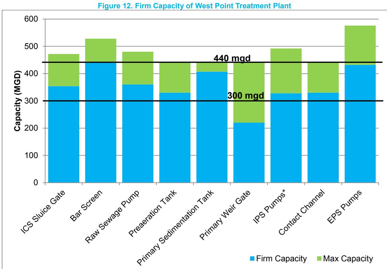
\* The IPS pumps do not need to meet the rated plant capacity of 440 mgd, as any flows greater than 300 mgd will be diverted around the secondary process via gravity.
