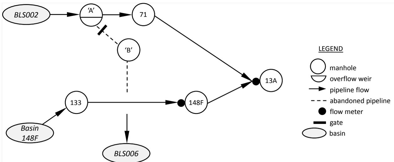
Figure 2-4. Skyway Post- I/I Demonstration Configuration (current)
