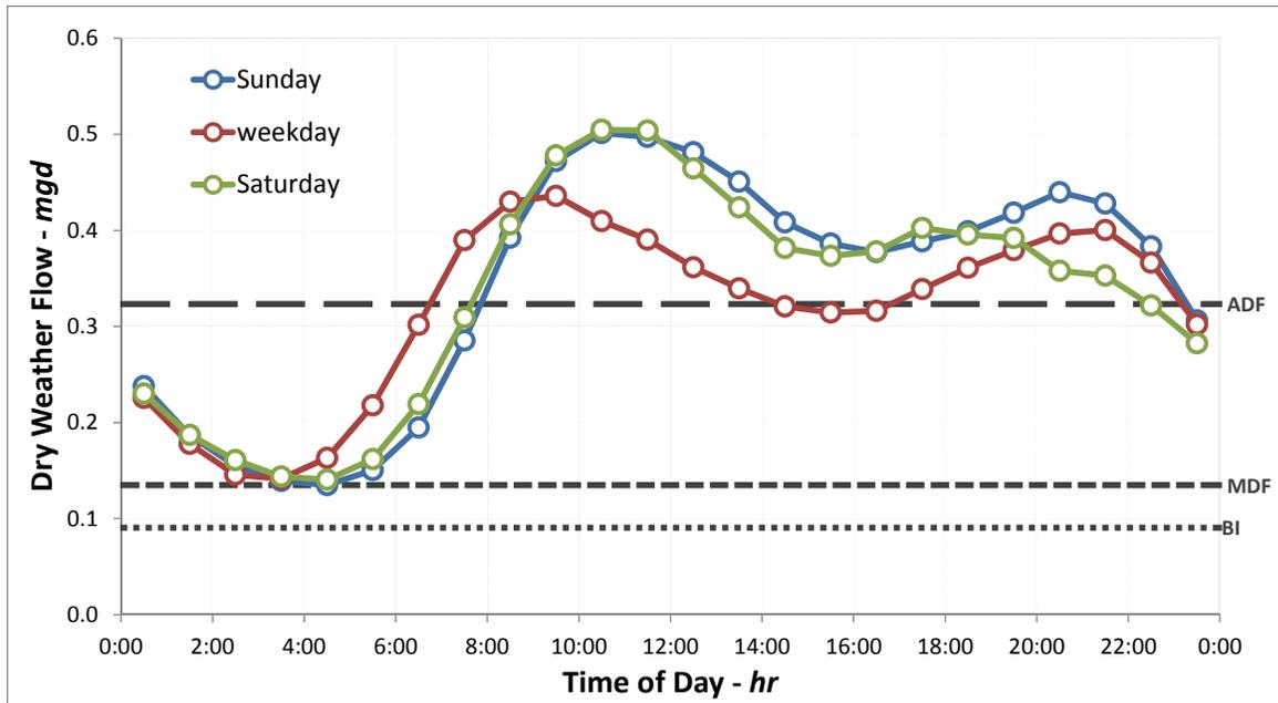
Figure 2-6. Example Dry-weather Flow Components and Diurnals
