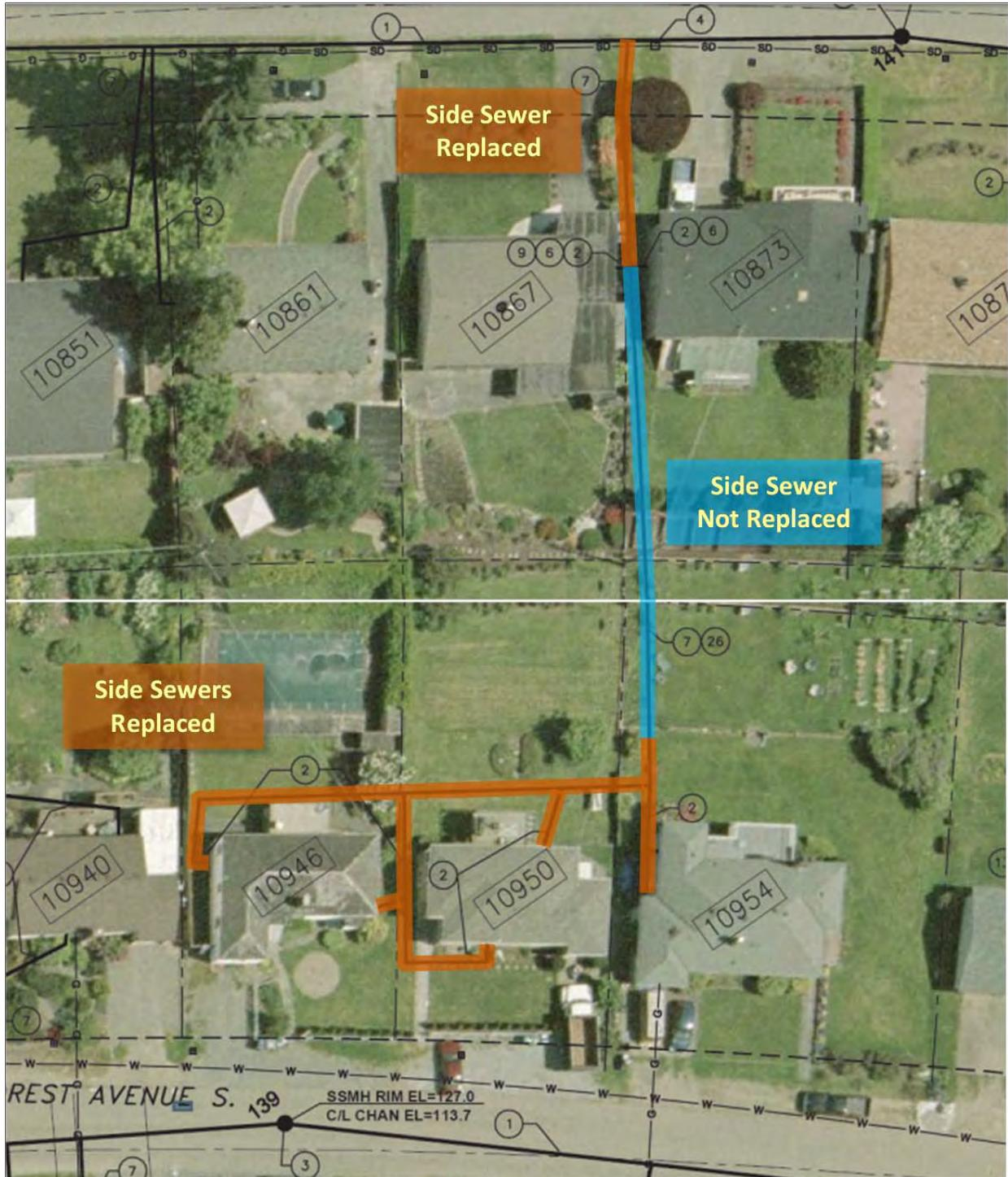
Figure 3-6. Partial Side Sewer Rehabilitation as Constructed
