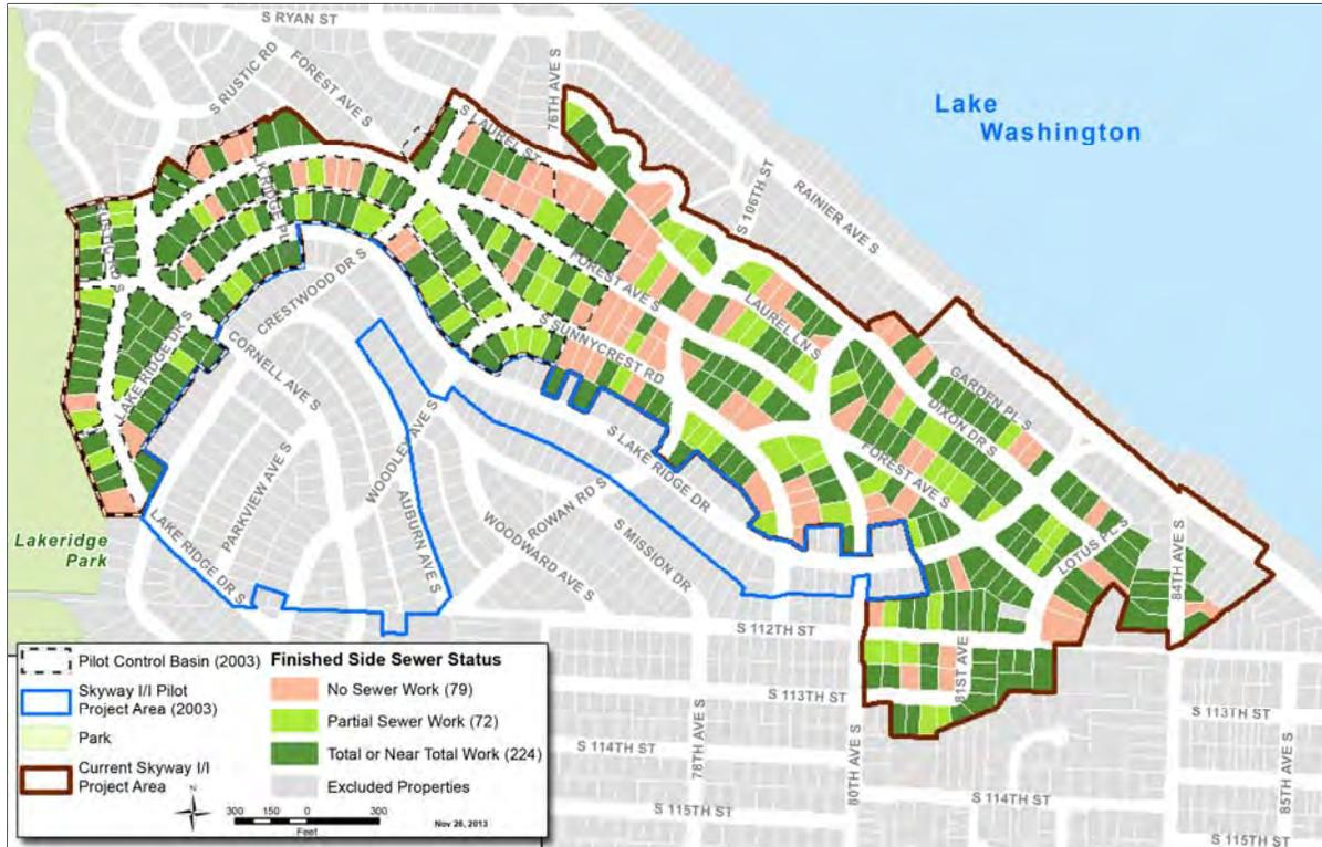
Figure 3-4. Side Sewer Replacement Status
