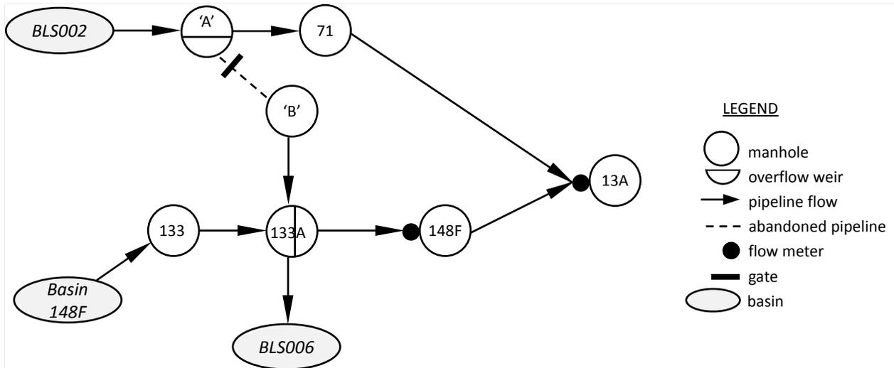
Figure 2-3. Skyway Post- I/I Pilot Configuration (interim)
