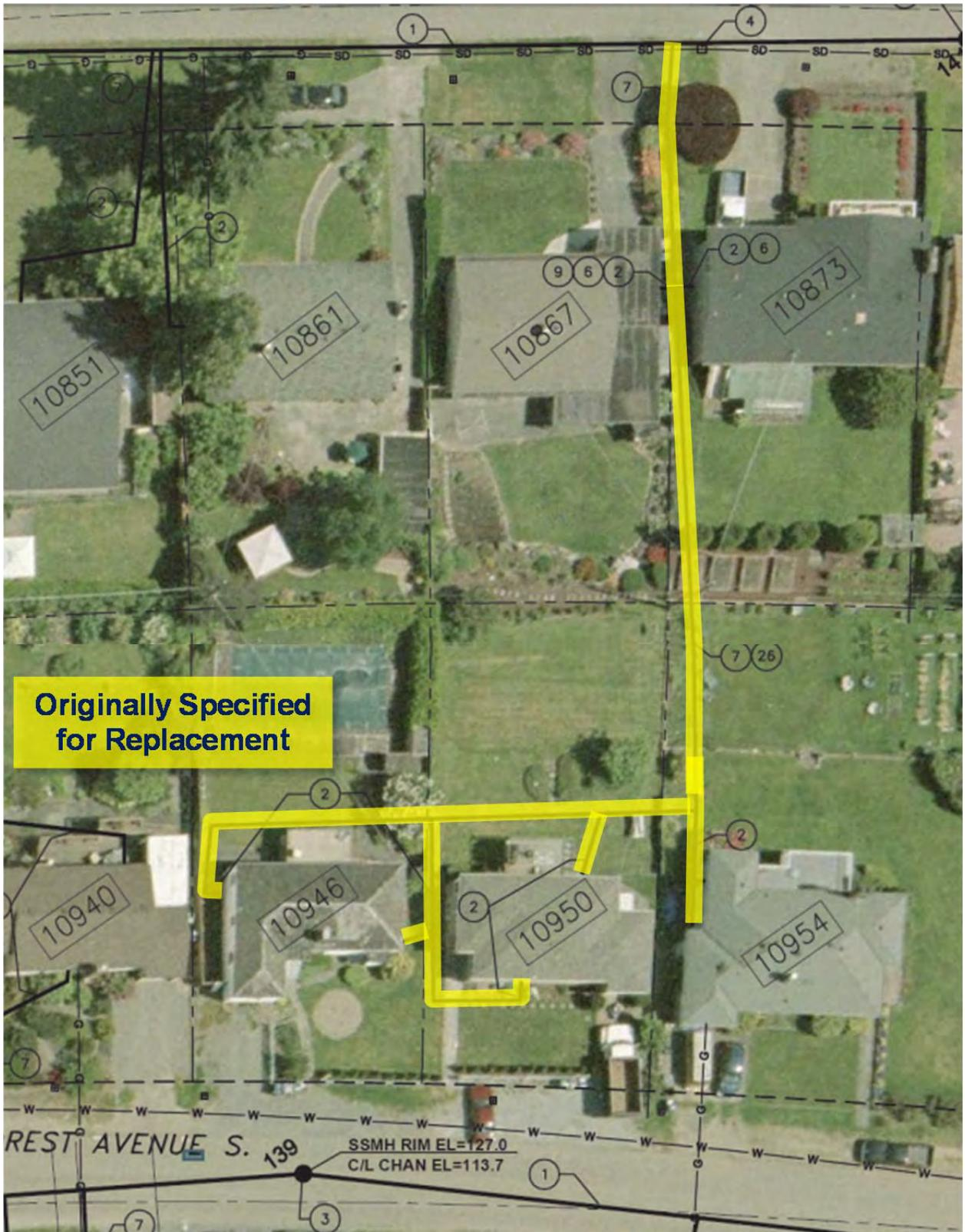
Figure 3-5. Full Side Sewer Rehabilitation as Designed
