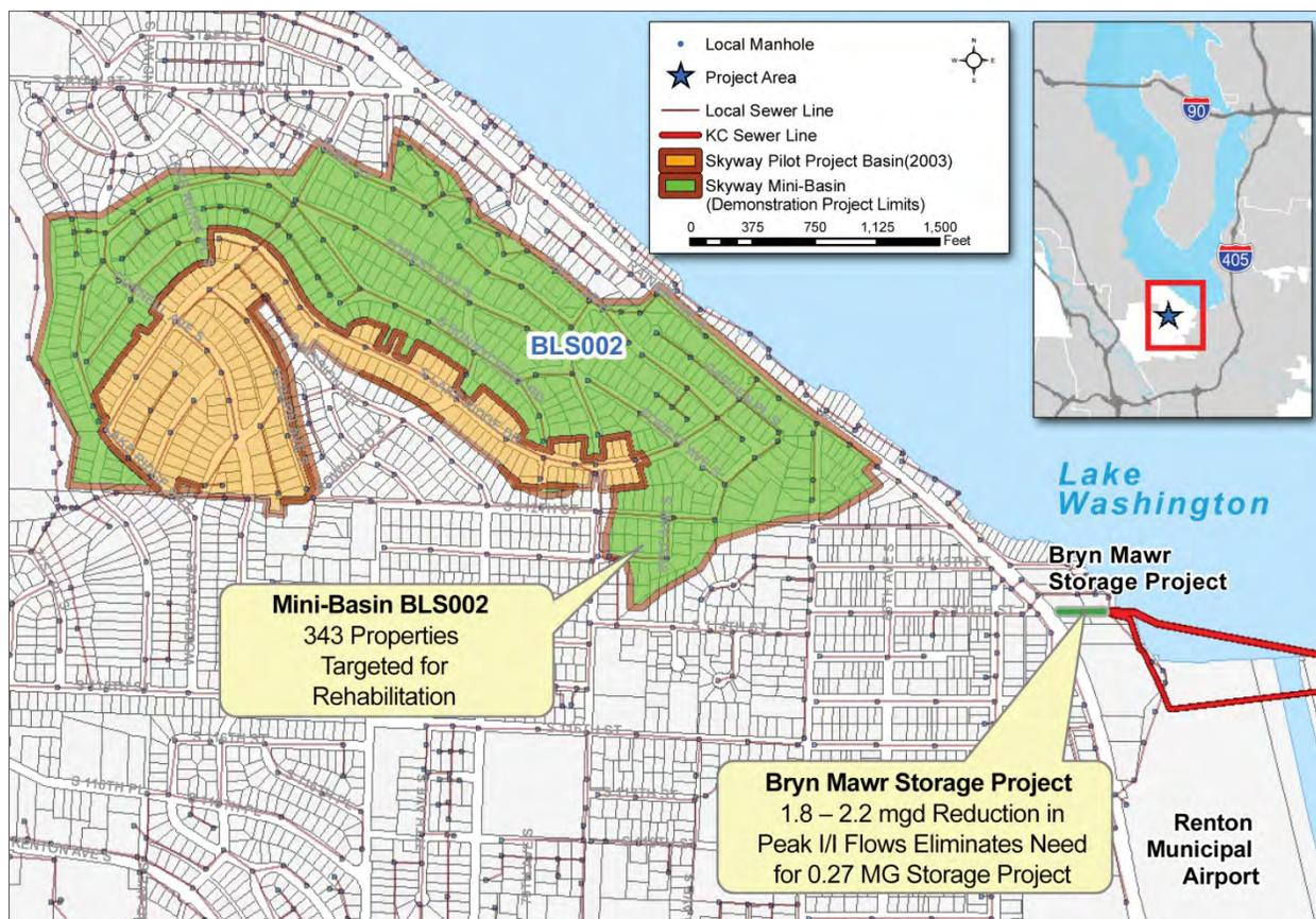
Figure 1-2. Skyway I/I Reduction Demonstration Project Location
