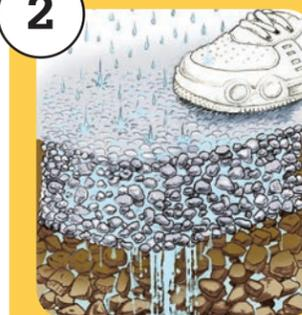
Permeable pavement is hard but porous material that allows stormwater to soak through into the ground below. Bicycles and cars can travel on permeable pavement.
