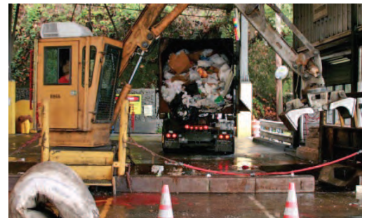
Commercial and self-haul customers dump directly into the refuse trailers located in the trailer tunnel, under the chutes, from the tipping floor above. A stationary compactor is used to distribute and tamp the material in the trailer.
