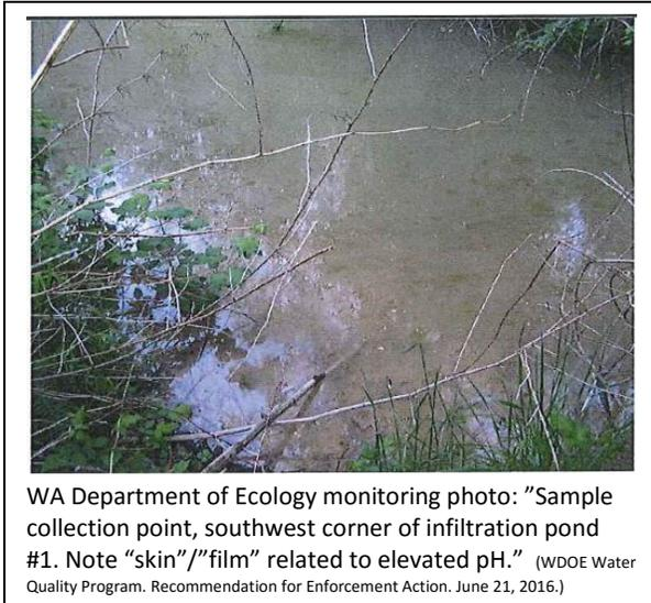
WA Department of Ecology monitoring photo: "Sample collection point, southwest corner of infiltration pond #1. Note "skin"/"film" related to elevated pH." (WDOE Water Quality Program. Recommendation for Enforcement Action. June 21, 2016.)
