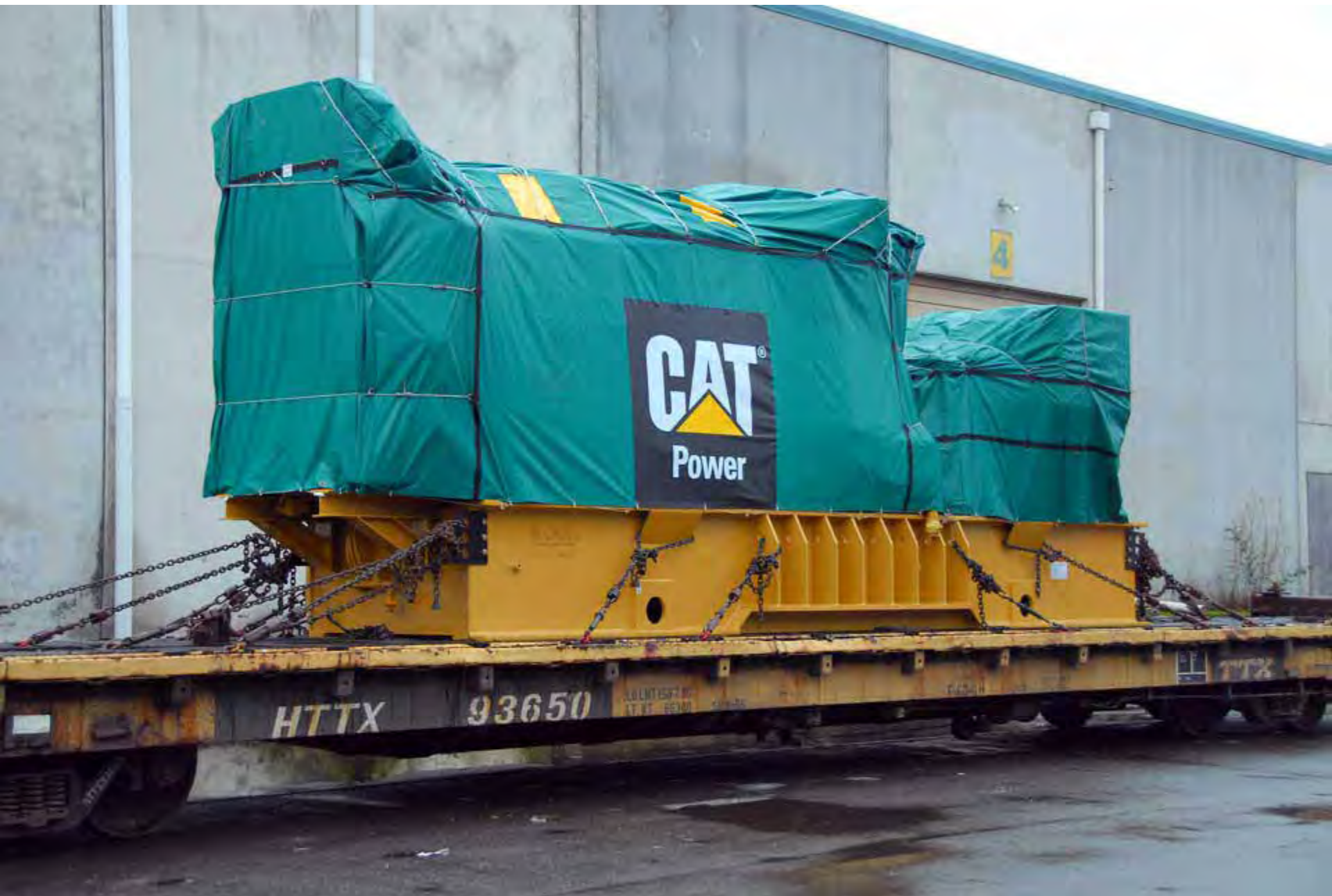
One of the 2.3 megawatt engine generators
