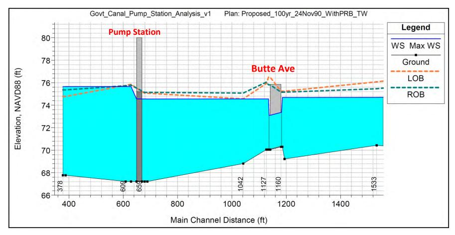
Figure 5 – Modeled water surface elevation profile (feet, NAVD88) in lower Government Canal during a 100-year event, with the pump station
