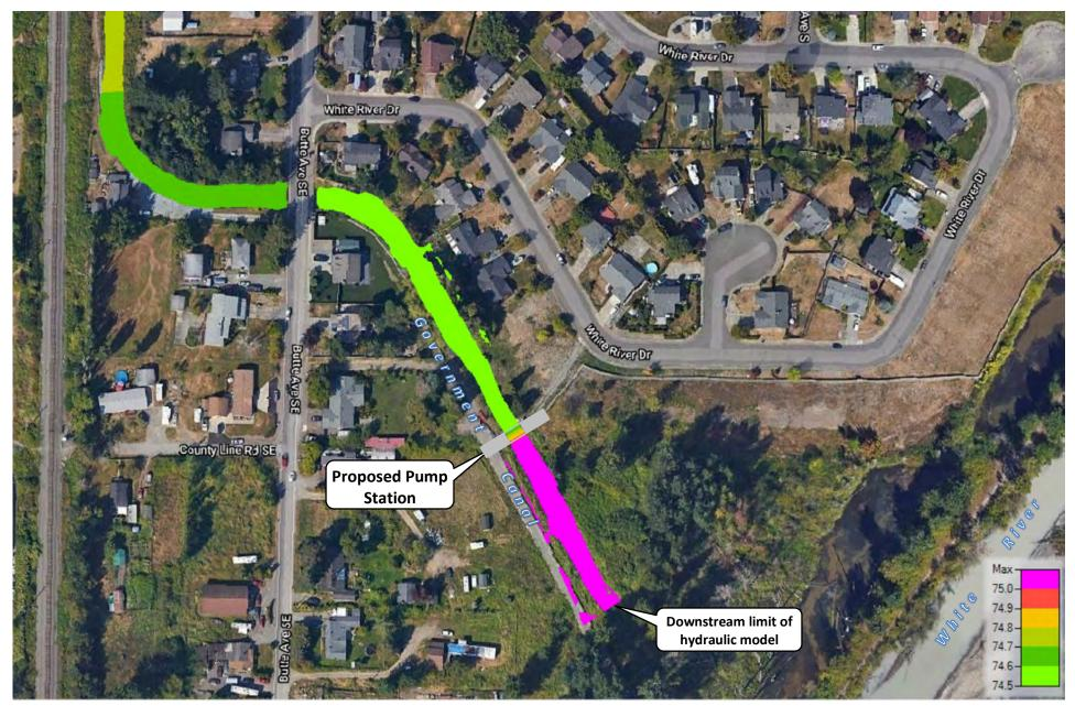
Figure 6 – Simulated water surface elevation (feet, NAVD88) and extent of flooding along Government Canal during a 100-year event, with the pump station
