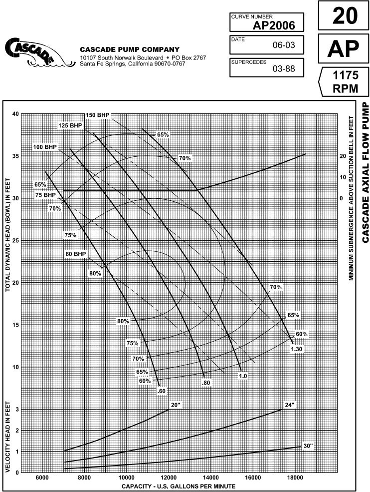
CURVE CHARACTERISTICS BASED ON PUMP PERFORMANCE WITH SPECIFIED AMOUNT OF CLEAR, NON-AERATED, FRESH COLD WATER.
