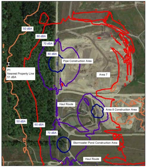
Figure 1. Sound Level Isopleths - Nearest Construction to P1
