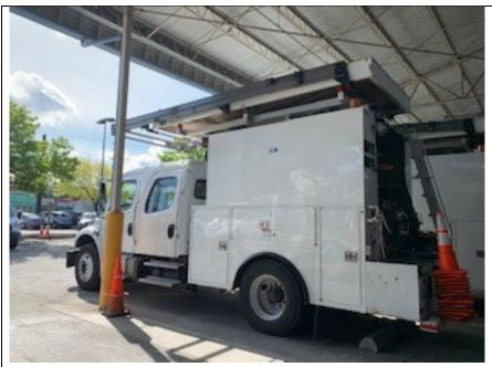
Fiberglass floored platform/lift truck. Safety railings on platform are manuallly lifted in to place with 50 lbs. of force. Platform is accessed via rear fixed ladder.
